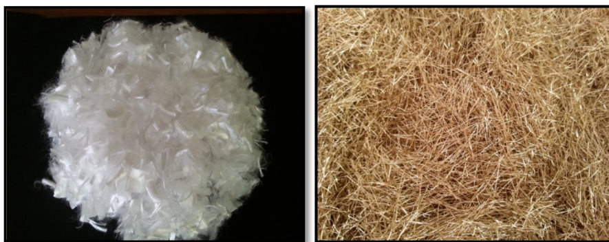
Plate (1) polypropylene fibers (left) and steel fibers (right)
