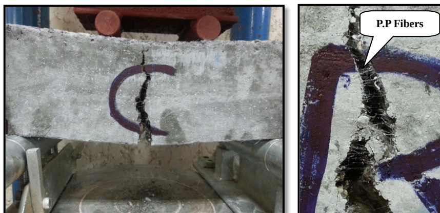
Plate (3): Flexural strength of high strength concrete
